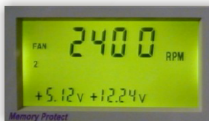
Fig.3 LCD Display - Back-light On - Scan Mode
